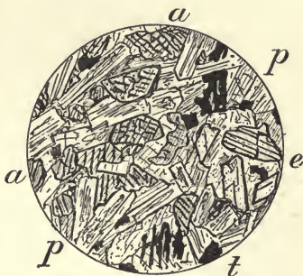
Fig. 29.—Altered Dolerite (Diabase). Mynydd-y-Gader, Cader Idris, N. Wales. \times 24 . a , Characteristic pale-brown augite. e , Almost colourless epidote, associated with pale chloritic areas, in which it crystallises out, giving elongated sections. p , Prismatic plagioclase. t , Titanic iron ore.
